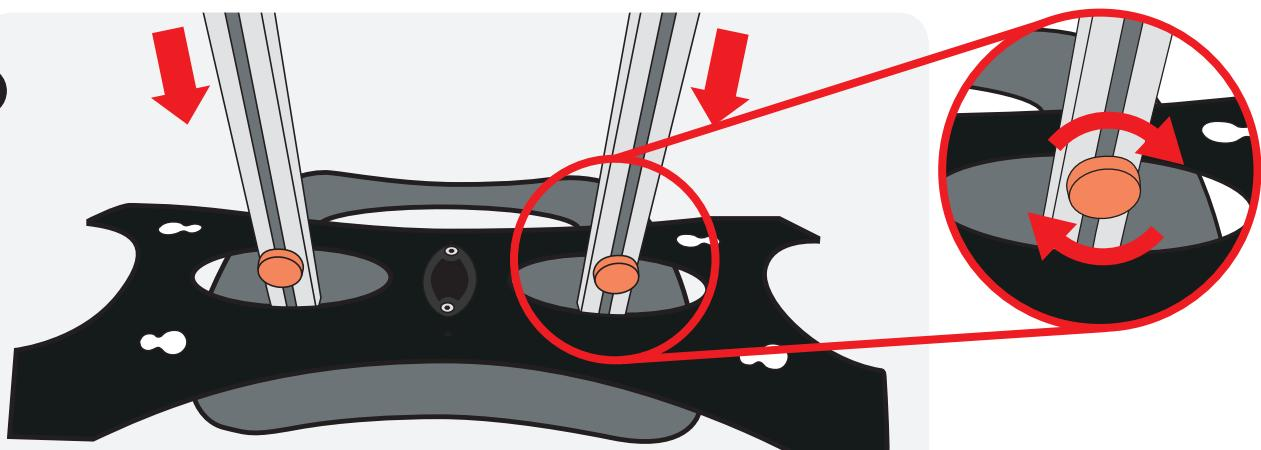
Slide the bottom AV uprigths (orange fixing) on to the AV base, and tighten the orange screws.
