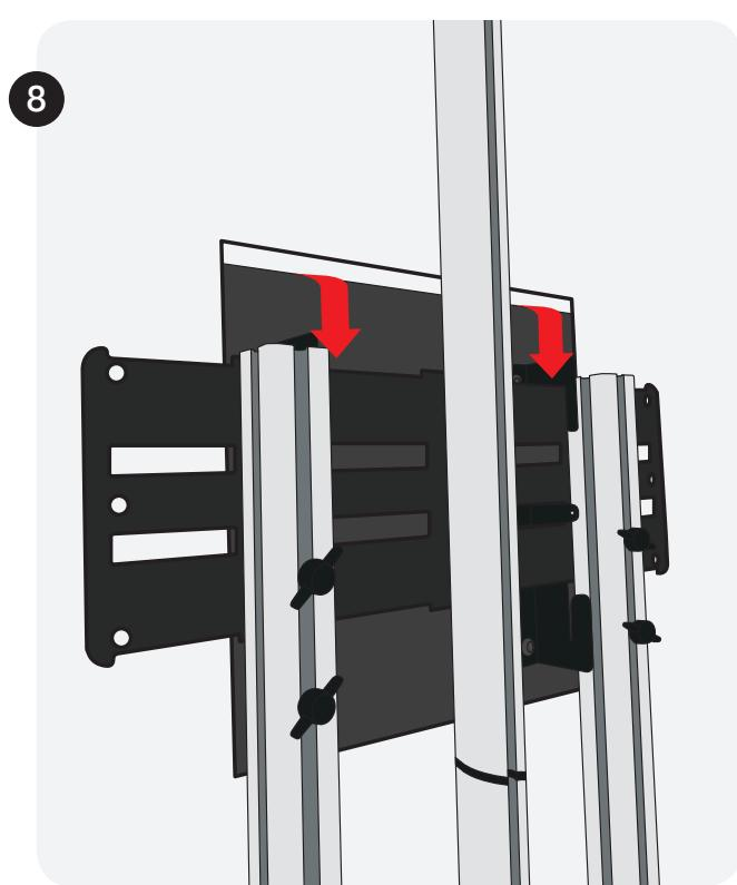
Once you have attached the brackets provided to the TV/Monitor screen, manoeuvre the screen into position so that the two brackets sit on top of the crossbeam. Once the screen is in position, further alterations can be made for cables if required.
