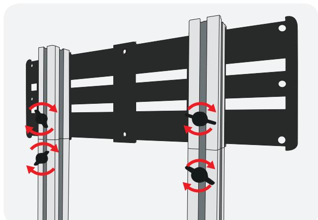
Locate the AV crossbeam into position and tighten the locking pins.
