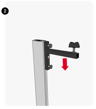
Insert iPad arm into the middle TWIST extrusion. Loosely tighten one of the screws to stop it falling down the complete extrusion.
